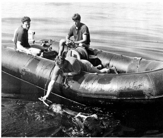
SEA LION prepares to grab mouthpiece he will attach to submerged ASROC. Spring-loaded clip on mouthpiece is jammed by animal over U-bolt on tail of weapon. Note line and spool; after clip is attached, test unit is hauled up. Men are Navy personnel assigned to Project QuickFind.
